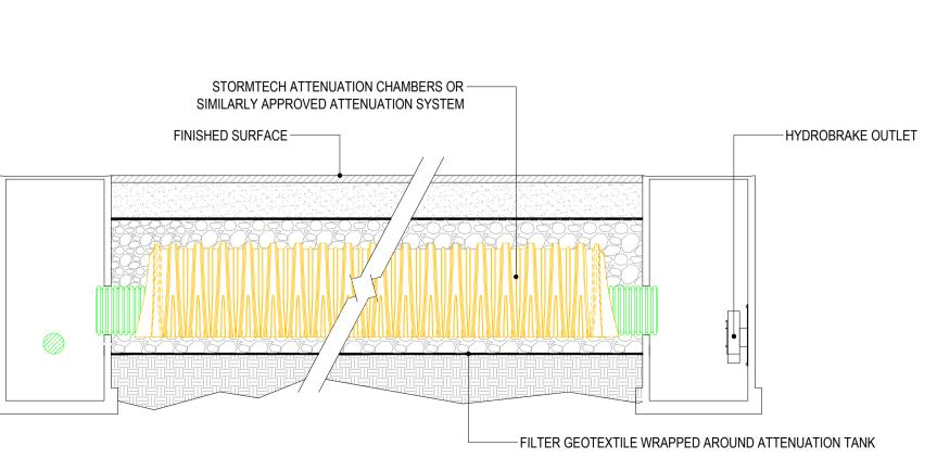
TYPICAL ATTENUATION TANK Scale: 1:50
